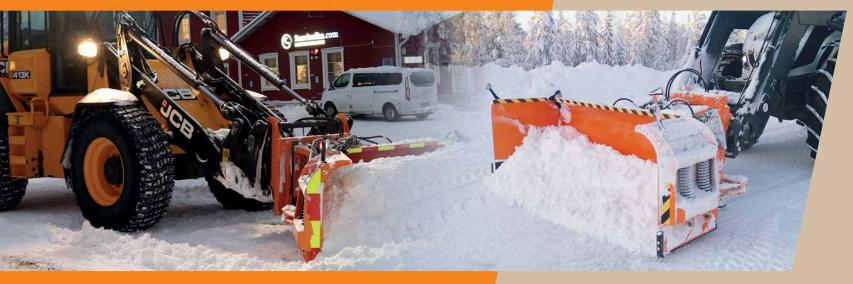
FMG U-plough is really multiuse plough. It is combination of bulldozer blade, articulated plough and collecting plough. U-plough consists of main wing and two flipper wings and the turning angle of side wings are even 175 degrees. The plough is the most popular, especially in wheel loaders use.
