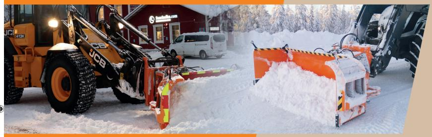
FMG U-plough is really multiuse plough. It is combination of bulldozer blade, articulated plough and collecting plough. U-plough consists of main wing and two flipper wings and the turning angle of side wings are even 175 degrees. The plough is the most popular, especially in wheel loaders use.
