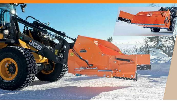
Hybrid bucket is FMG's patented equipment, that is combined as a flipper bucket and ice-removing bucket. Due to the special structure Hybrid bucket works as flipper bucket so that the ice-removing blade does not catch the ground. When the bucket is tilted back so that the cutting edge rises from the ground, the ice-removing blade starts to remove the ice. The removed ice is getting into the bucket and ready to be tipped onto the bench.
