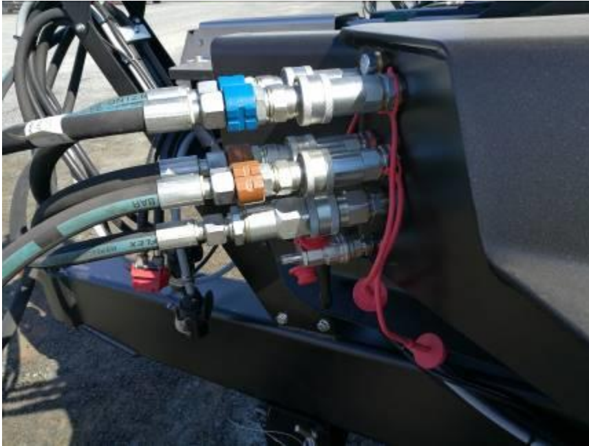
Picture 25. Hydraulic couplings are connected to hose rack
