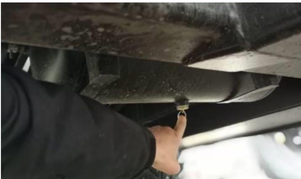
Picture 34. Condensation water removal from air pressure container
