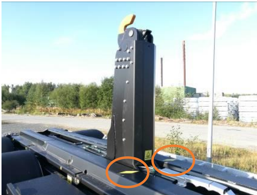
Picture 24. Hook tower in middle position
