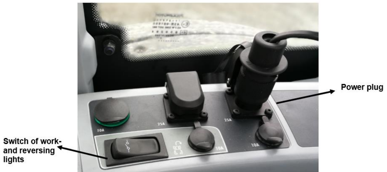
Picture 31. Connection of work- and reversing lights and connection of control system to the tractor
